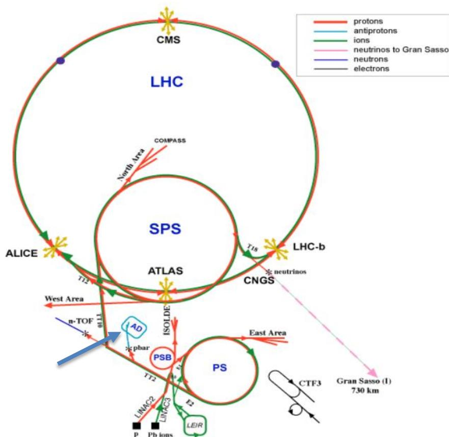
The access point for AD is located building 193, which is located in front of the Booster (PSB). It consists of a total of 189 magnets powered by some 110 power converters. There is one central supply for the Dipoles (with 12 adjusting trimmers) and two central supplies for the Quadrupoles (with 5 adjusting trimmers). A pair of two other magnets (in TT2 and Sector 4) are powered in series by two power converters while all remaining magnets are powered by a dedicated power supply.
